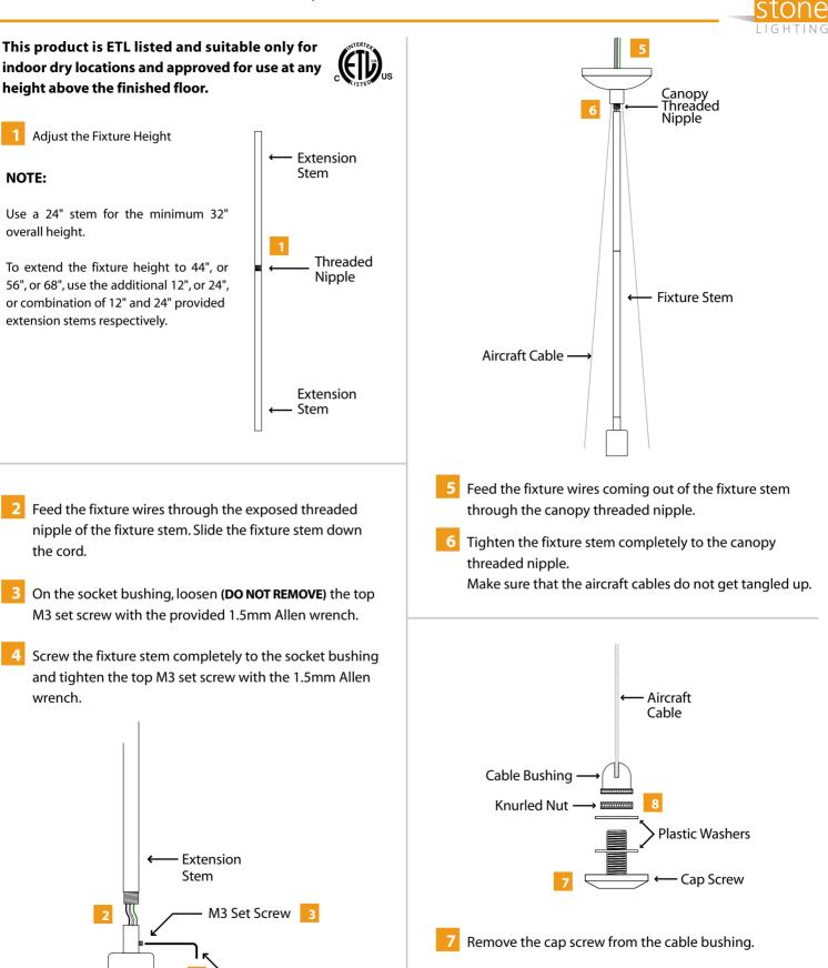
8 Remove the knurled nut and one of the plastic washers from the cap screw.
